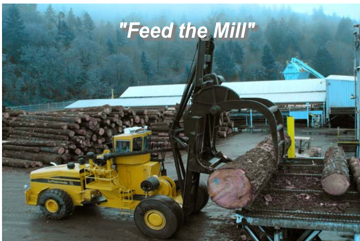
"Environmentally Friendly, No Hydraulic Cylinders to Leak & Pollute the Water"
